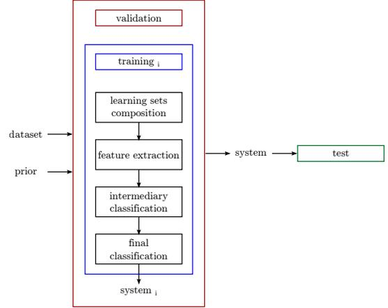
Fig. 3: Learning. Multiple training instances  $i$  are launched, each one resulting in a classification system  $i$ . These systems are evaluated through validation and one is selected for test. The inputs are the dataset and the prior, while the outputs are the selected system together with its test evaluation.
