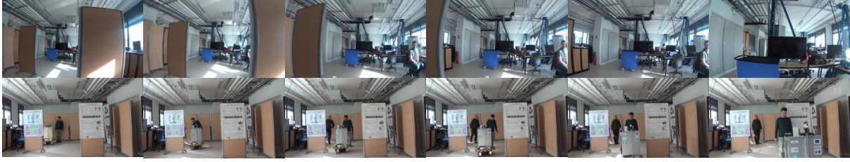
Fig. 7. Real experiment with our MPO700 platform navigating towards a blue chariot. Top: images from the on-board camera, bottom: robot behaviour while avoiding two obstacles.
