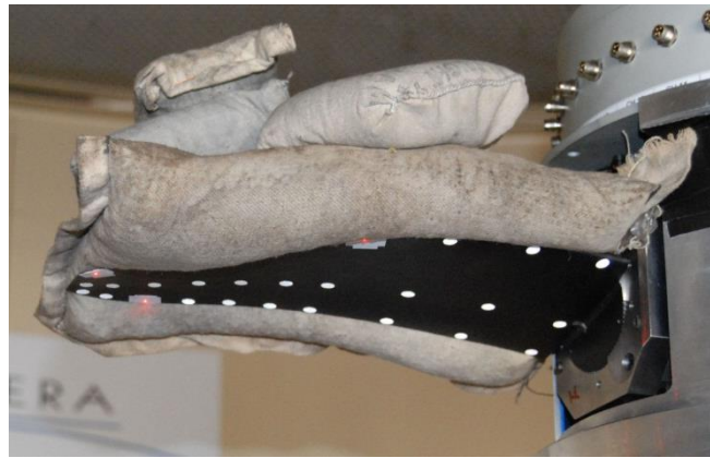
Figure 8 - Distributed loading for rear blade static validation
