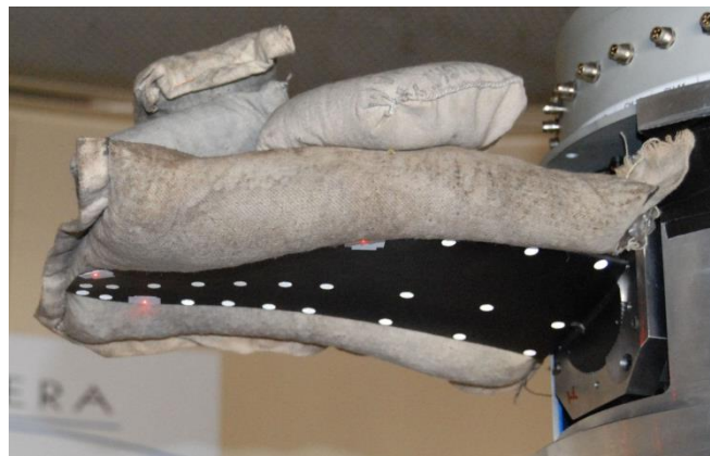
Figure 8 - Distributed loading for rear blade static validation
