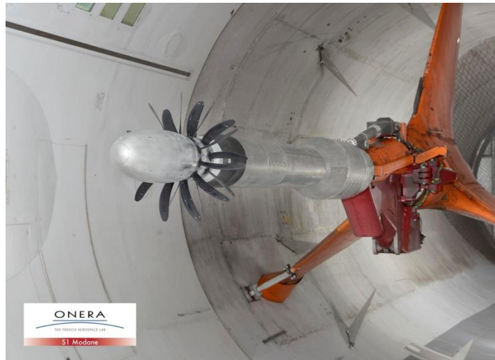
Figure 1 – Z49 CROR in ONERA S1MA WTT
