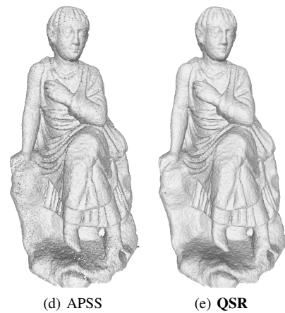
Figure 8: Groundtruth Comparison: super-resolution of an artificially degraded shape. The degradation involves a subsampling to 10% of the points and an additional Gaussian noise of variance 0.005% of the diagonal. Processing radius: r = 0.2 (Shape diagonal: 23.83), nbins_{lr} = 25 , nbins_{sr} = 100 , r_{sim} = 0.05 . Normals are computed using PCA with 10 neighbors for visualization purpose.
