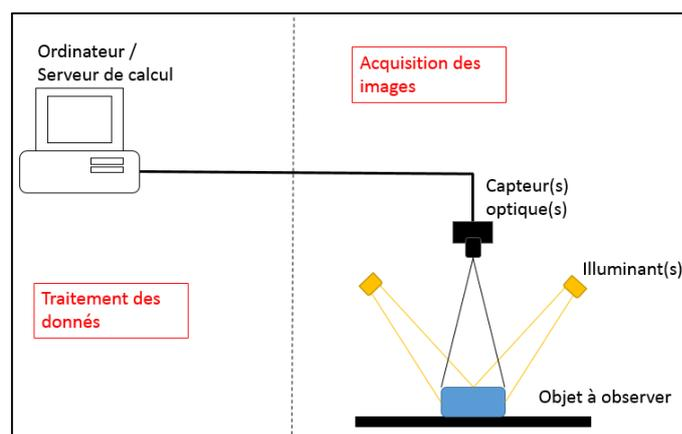
Figure 1. COMPOSITION SIMPLIFIEE D'UN SYSTEME D'INSPECTION AUTOMATISE
