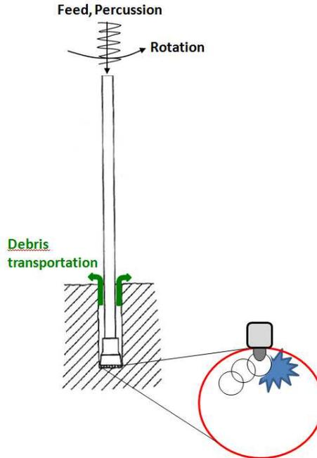
Figure 5. Schematic picture of real rock drilling.
