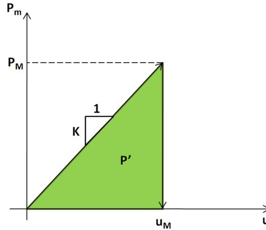
Figure 7. Idealized stress-deformation curve during percussive action ([3, 13]).
