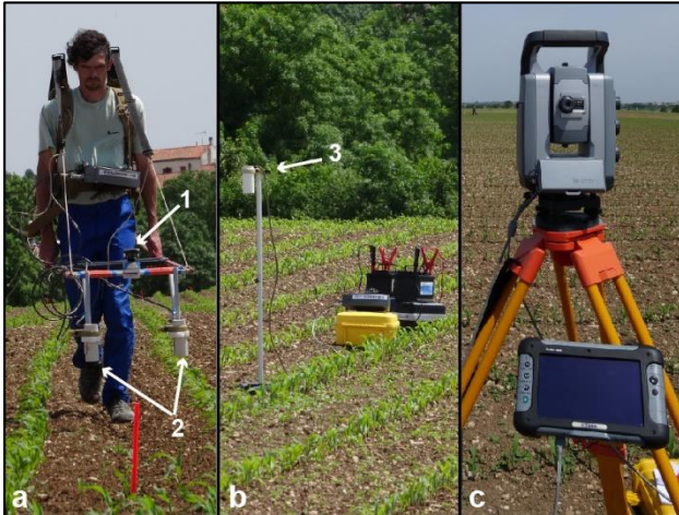
Fig. 2. a: G-858 magnetometer (Geometrics) with two caesium vapour sensors, horizontally spaced 0.39m apart (2). Glass prism reflective placed between the two sensors (1). b: G-858 magnetometer disposed in base-station (3). c: motorised total station (S8, Trimble).
