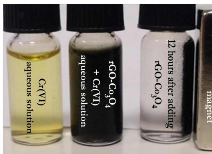
**Figure 8:** Images of Cr(VI) adsorption by rGO-Co<sub>3</sub>O<sub>4</sub> nanocomposite and magnetic recovery of the catalyst by application of an external magnet (1 Tesla).
