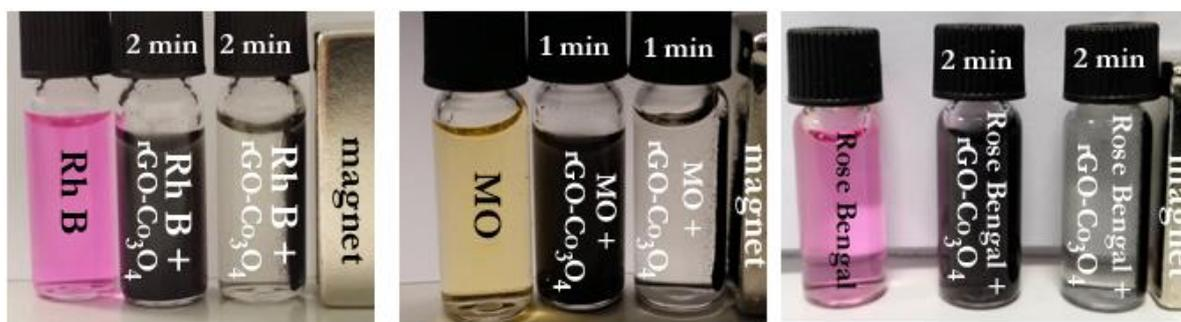
**Figure 12:** Photographs of (A) RhB, (B) MO and (C) Rose Bengal aqueous solutions (5  $\mu\text{M}$ ) before and after treatment with 1 mg/ml of rGO-Co<sub>3</sub>O<sub>4</sub> nanocomposite. External magnet of 1 Tesla.
