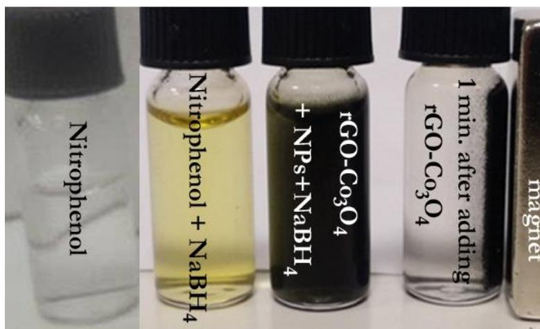
**Figure 6:** Images illustrating the catalytic reduction of 4-NP to 4-AP using rGO-Co<sub>3</sub>O<sub>4</sub> nanocomposite as catalyst and its separation at the end of the process using an external magnet.
