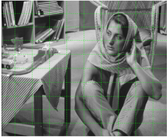
(a) Reference image ( 1151 \times 1407 pixels) with 9 \times 9 grid points (overlaid in green) where PSFs are sampled.
