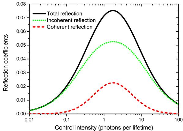
Figure 6. **Ideal probe reflectivity in the population switch case.** The computed reflectivity of a vanishingly weak probe laser (tuned on the upper transition) is plotted as a function of the control laser power (tuned on the lower transition) in a copolarized situation with ideal parameters ( $\varepsilon = \Gamma/\gamma = 1$ ). The probe power is  $10^{-3}$  photon/lifetime. It can be observed that the reflection is mainly incoherent.
