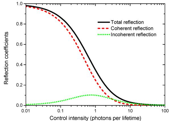
Figure 7. **Ideal probe reflectivity in the Autler-Townes configuration.** The computed reflectivity of a vanishingly weak probe laser (tuned on the lower transition) is plotted as a function of the control laser power (tuned on the upper transition) in a copolarized situation with ideal parameters ( $\varepsilon = \Gamma/\gamma = 1$ ). The probe power is  $10^{-3}$  photon/lifetime. The reflectivity is mainly coherent and reaches unity at low control laser power.
