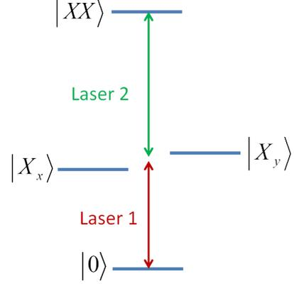
Figure 4. **Level scheme.** Levels  $|X_x\rangle$  and  $|X_y\rangle$  are the two fine structure split excitonic eigenstates. In practice they are separated by  $25 \mu\text{eV}$ , and we can consider only one of them. Level  $|XX\rangle$  corresponds to the biexciton. Laser 1 (2) is tuned around the lower (upper) transition.
