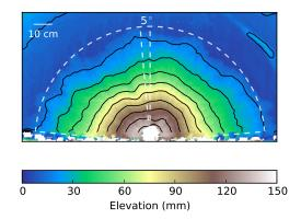
**Figure 6.** Digital elevation model of an experimental fan (run 2). Black lines: elevation contours 15 mm apart from each other. White dashed lines indicate the bounds used for averaging (only two sample radii  $5^{\circ}$  apart are represented for clarity).
