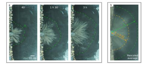
**Figure 3.** Top-view pictures of an experimental fan (run 2). (a) Time evolution. Green dashed line indicates fan toe,  $R_c$ . (b) Average of rescaled pictures. The 26 pictures are each 10 min apart. Dashed lines indicate silica–coal transition (orange) and fan toe (green). After rescaling, the fan length is 1. Transition between silica and coal occurs at dimensionless distance  $\mathcal{R}$  from apex.
