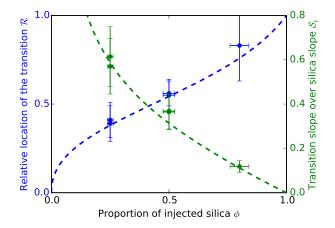
**Figure 14.** Relative position of the transition  $\mathcal{R}$  (blue) and dimensionless transition slope  $\mathcal{S}_t$  (green), as a function of the composition of the sediment input. Dots: experimental measurements. Dashed lines: Eqs. (9) and (10) with  $\mathcal{S} = 3.4$ .
