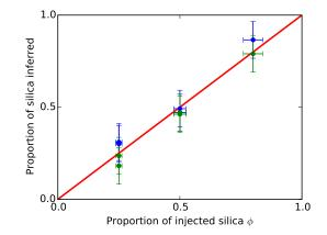
**Figure 10.** Proportion of silica inferred from the geometry of the deposit, after Eq. (9) (blue) and after Eq. (10) (green), as a function of the composition of the sediment input. Red line: perfect agreement.
