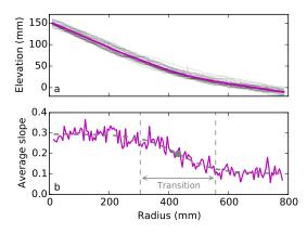
**Figure 7.** (a) Fan profiles at different angles (run 2). Gray: individual profiles; magenta: average profile. (b) Average downstream slope (magenta). Fitted hyperbolic tangent (dashed gray). Inflection point (gray dot) and boundaries of the transition area (vertical dashed gray lines).
