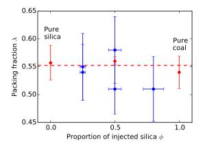
**Figure 5.** Packing fraction of the deposit as a function of the composition of the sediment mixture. Blue dots calculated from experiment. Red dots measured independently. The red dashed line is the mean packing fraction measured independently.
