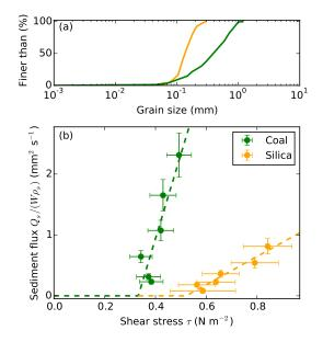
**Figure 2.** (a) Cumulative density function of the grain size. Orange: silica; green: coal. (b) Transport laws. Volumetric flux per unit width, as a function of dimensional shear stress. Dashed lines correspond to Eq. (A3) fitted to the data (method in Appendix A; coefficients in Table 1).
