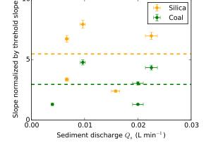
**Figure 13.** Slope normalized by the threshold slope, calculated with Eq. (11), as a function of the sediment discharge. Dashed lines: average slopes.
