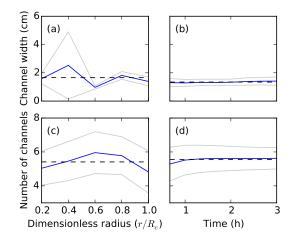
**Figure 12.** Evolution of active channels for all the runs. Channel width as a function of the dimensionless radius (**a**) and time (**b**). Number of channels as a function of dimensionless radius (**c**) and time (**d**). Black dashed line: average. Gray lines: variability over experimental runs.
