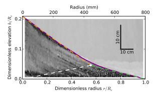
**Figure 8.** Average radial profile (magenta line), superimposed on radial cross section, for run 2. Dashed lines: slope of the silica (orange) and coal (green) deposits. White dashed line indicates silica– coal transition. Scale is for the picture. h and r are, respectively, the fan elevation and the distance to the apex.
