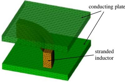
Fig. 7. Stranded inductor and two conducting plates.
