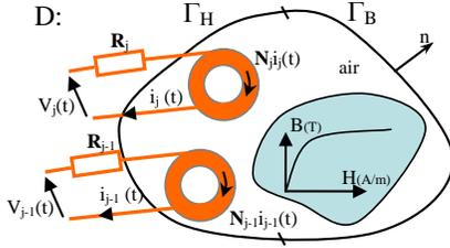
Fig. 1. Non-linear magnetostatic problem coupled with electric circuits.
