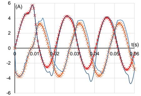
Fig. 6. Evolutions of the current associated with two primary windings for resistor load (R=200Ω).
