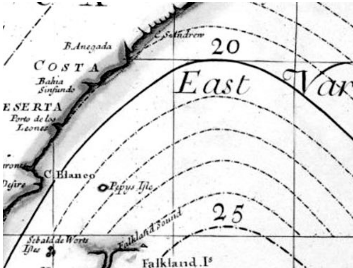
Figure 5: Detail of a so-called “isogonic” map produced in 1701 by Edmond Halley and believed to be first data-based contour map showing lines of equal magnetic declination (Friendly, M. & Denis, D. J. (2001). Milestones in the history of thematic cartography, statistical graphics, and data visualization. Web document, http://www.datavis.ca/milestones/ ).
