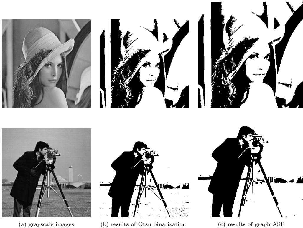
Fig. 11 Illustration of Otsu binarization followed by mathematical morphology filtering on graphs from two images of the Standard image dataset.
