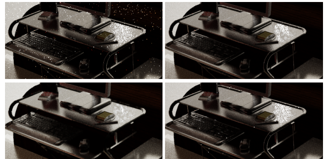
Figure 2: Top left: original, right: final despeckled image. Bottom left: without clusterization. Note that the borders of the table have been considered as speckles and therefore reconstructed. Right: clusterization without using a threshold ratio. Note that speckles that lie on the table border are still present, as they are part of the border cluster.
