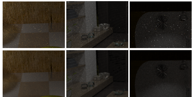
Figure 5: Top row: close-up on original HDR images, using a low exposure value for the tonemapping to make high-frequency/large-amplitude noise more visible. Bottom row: after processing with our method.
