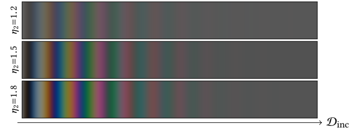
Fig. 11. The Airy reflectance term at normal incidence is visualized for \mathcal{D}_{\text{inc}} \in [0..6400]\text{nm} with three values of \eta_2 (one per row); other material parameters are held fixed to \eta_3 = 1.1 and \kappa_3 = 1.5 . Color saturation and intensity increase with larger values of \eta_2 .
