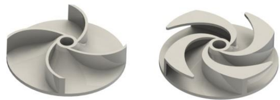
Figure 2. Schematic view of the impellers of a vortex pump without winglets (left) and with winglets (right)
