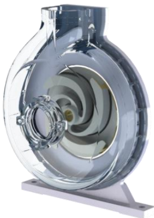
Figure 1. Schematic view of a vortex pump with recessed impeller and enlarged front chamber
