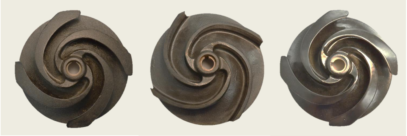
Figure 4 Impellers of study 2: Impeller with winglets and casting surface (left), semi-open impeller (without winglets, middle), impeller with winglets and smoothed surface (right)
