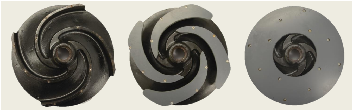
Figure 3 Impellers of study 1: Semi-open impeller (left), impeller with winglets (middle), impeller with front shroud (right)
