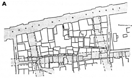
A. Portion of Tanjore Fort. The Municipal Council's proposals for the relief of congestion. Cost about Rs 30,000. Scale 1 cm. equals 100 feet.
