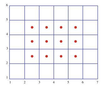
**Fig. 18.** The index space corresponding to the biquadratic B-spline surface seen in Fig. 16. The anchor for each function is shown as a red circle. For this even-degree case (p=2), the anchors fall in the centers of the cells. For an odd polynomial degree, the anchors would fall at the intersections of knot lines. Note that, regardless of degree, an anchor falls at the center of the support of a function in the index space.
