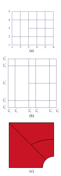
**Fig. 26.** T-mesh and its images in the parameter and physical spaces for a plate with a circular hole. (a) T-mesh in the index space. (b) T-mesh in the parameter space. (c) T-mesh in the physical space.
