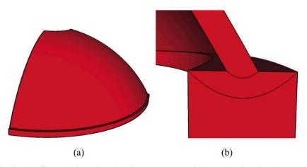
Fig. 49. Hemispherical shell with stiffener. Initial T-mesh in physical space, NDOF = 360: (a) Coarse T-mesh in physical space and (b) detail of stiffener.
