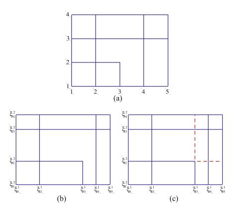
**Fig. 29.** Valid T-meshes for splines of odd polynomial degree can have L-junctions. The rules for inferring local knot vectors are in no way changed for such a structure. (a) Example of a T-mesh in index space with an L-junction and p = 3. (b) T-mesh in the parameter space. (c) Elements are defined by the union of the knot lines and the continuity reduction lines.
