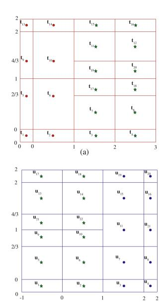
Fig. B.5. Local refinements of T-meshes from Fig. B.4 to arrive at matching patches. Control points of anchors designated by stars are adjusted such that the boundaries of the two geometries match.
