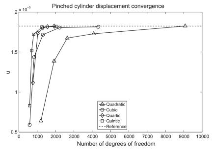
Fig. 47. Shell obstacle course. Pinched cylinder displacement convergence.
