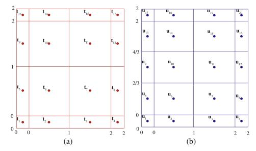
Fig. B.1. T-meshes in parameter space and knot values of two quadratic NURBS patches. In this figure, anchors are designated by red and blue circles.
