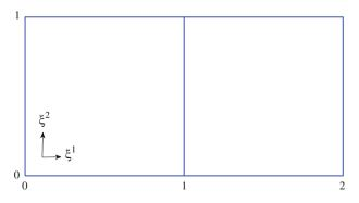
**Fig. 17.** The domain of the mesh, a subset of the parameter space, corresponding to the biquadratic B-spline surface seen in Fig. 16. The domain of the mesh is the preimage of the physical mesh.
