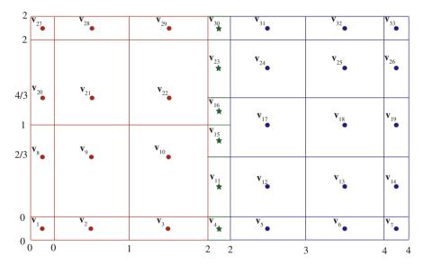
**Fig. B.3.** Merged  $C^0$  geometry represented by a single T-mesh.
