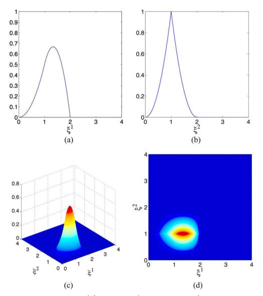
Fig. 15. Bivariate quadratic B-spline basis function  $B_{\{3,3\},\{2,2\}}(\xi^1,\xi^2)$  for knot vectors  $\Xi^1=\{0,0,0,1,2,2,3,4,4,4\},\Xi^2=\{0,0,0,1,1,2,3,4\}$ . (a) Univariate B-spline basis function  $N_{3,2}^1(\xi^1)$ . (b) Univariate B-spline basis function  $N_{3,2}^2(\xi^2)$ . (c) Tilted view of  $B_{\{3,3\},\{2,2\}}(\xi)$ . (d) Overhead view of  $B_{\{3,3\},\{2,2\}}(\xi)$ .
