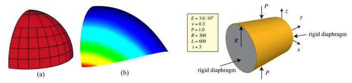
**Fig. 42.** Shell obstacle course. Pinched hemisphere with p=5, NDOF = 1524: (a) Tmesh in physical space and (b) displacement contours in direction of inward directed point load on deformed configuration (scaling factor of 30 used).
