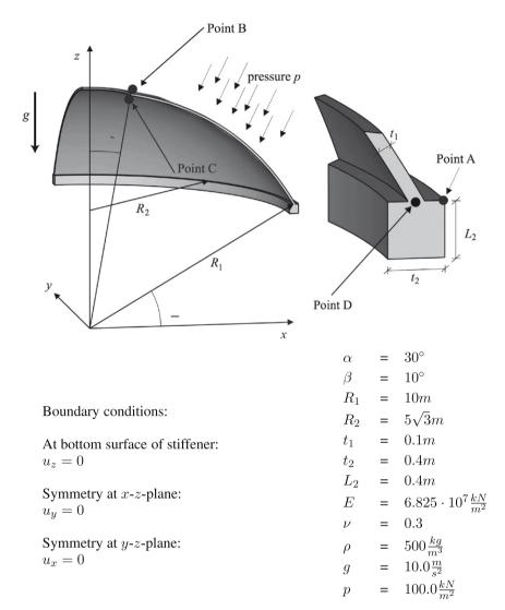
Fig. 48. Hemispherical shell with stiffener. Problem description from Rank et al. [39].
