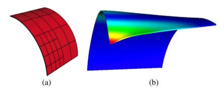
**Fig. 46.** Shell obstacle course. Pinched cylinder with p = 5, NDOF = 1260: (a) T-mesh in physical space and (b) displacement contours on deformed configuration (scaling factor of  $3 \times 10^6$  used).
