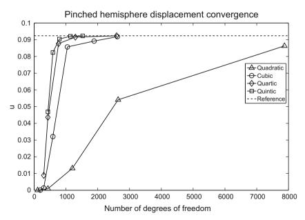
Fig. 43. Shell obstacle course. Pinched hemisphere displacement convergence.
