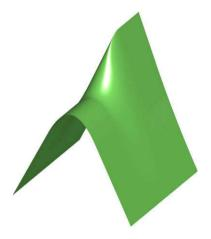
Fig. 27. T-splines allow continuity to change abruptly.
