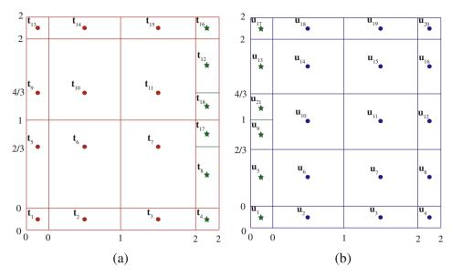
Fig. B.2. Local refinements of T-meshes from Fig. B.2 to arrive at matching patches. Control points of anchors designated by stars are adjusted such that the boundaries of the two geometries match.
