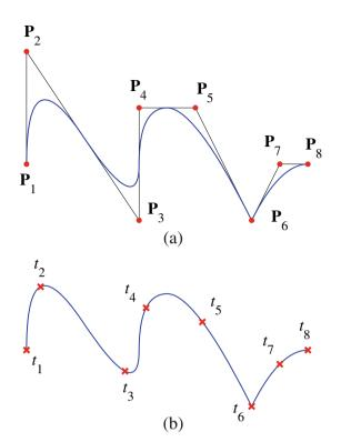
**Fig. 14.** Quadratic B-spline curve in  $\mathbb{R}^2$ . Knot vector and basis functions as in Fig. 12. (a) Curve with control points and control polygon. Control point locations are denoted by the red  $\bullet$ . (b) Curve with anchors. Anchor locations are denoted by the red  $\times$
