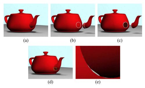
**Fig. 6.** Utah teapot model. (a) The original NURBS surfaces. (b) Intersection curves where the body and spout intersect (the spout has been moved away from the body). (c) Trimmed-NURBS representation in which the hole is cut in the body and the excess part of the spout is trimmed away. (d) Trimmed-NURBS body and spout moved back to their original positions. (e) Blowup showing the gap between the body and spout inside the green rectangle in (d).
