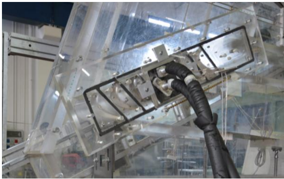
Figure 4. The cooling flow supply lines.
