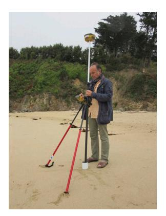
Figure 5. Backsight target accurately measured by RTK GPS, with GPS pole held by an adjustable bipod.
