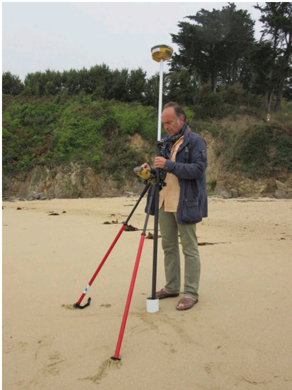
Figure 5. Backsight target accurately measured by RTK GPS, with GPS pole held by an adjustable bipod.
