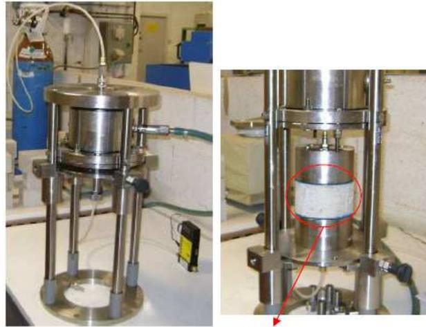
Cylindrical specimen Ø110 mm x H50 mm
