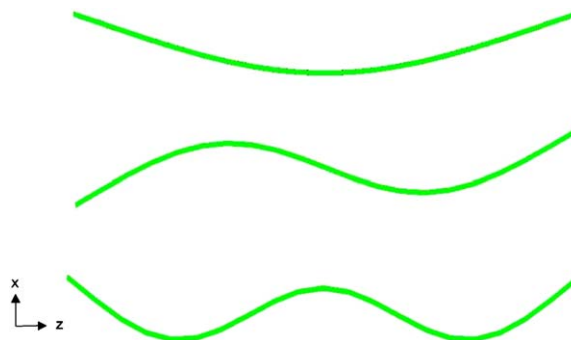
Fig. 57. NASA ATC. Selected calculated mode shapes for the stringer. Three lowest x - z modes.
