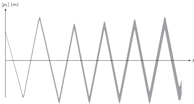
Figure 14: DAURADE’s tube [p_1](\cdot) computed as the primitive of [\dot{p}_1](\cdot) . This tube becomes thicker depicting cumulative uncertainties due to the dead-reckoning method. Observations pictured in Figure 12 are not represented here.
