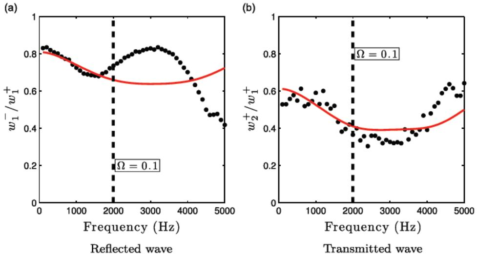
Fig. 8. Acoustic transfer functions. —: Analytical theory ; ○: Numerical simulations.
