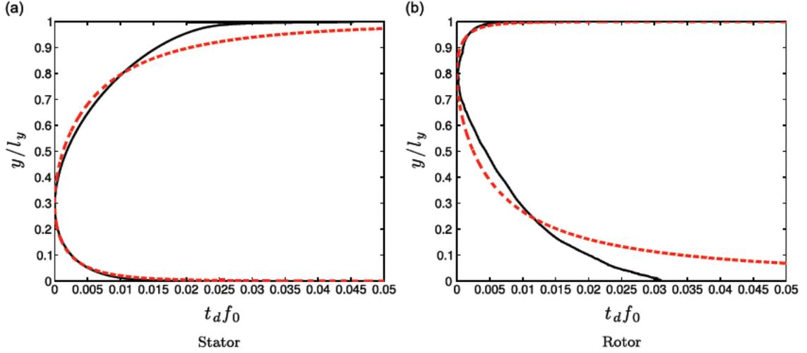
Fig. 12. Time-delay  $t_d(y)$  obtained using the LES mean flow (—), and a simplified analytical profile (---). Note that  $y/l_y = 0$  (respectively  $y/l_y = 1$ ) corresponds to the suction side (respectively pressure side) for the stator blade, and to the pressure side (respectively suction side) for the rotor blade.
