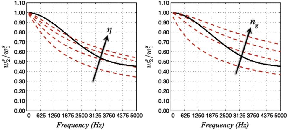
Fig. 13. A parametric study on the asymmetry ( $\eta = 0.1, 0.2, 0.3,$  and  $0.4$ , left) and flatness ( $n_g = 1, 2, 3,$  and  $4$ , right) of the velocity profile on the attenuation of the entropy transmission through this single row.
