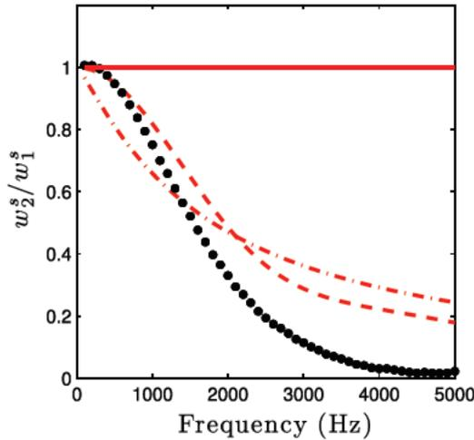
Fig. 10. Entropy transmission through the stator-rotor. —: Analytical theory without attenuation; ---: Analytical theory with attenuation extracted from the simulation; - . - .: Analytical theory with a simplified attenuation model ; ●: Numerical simulations.
