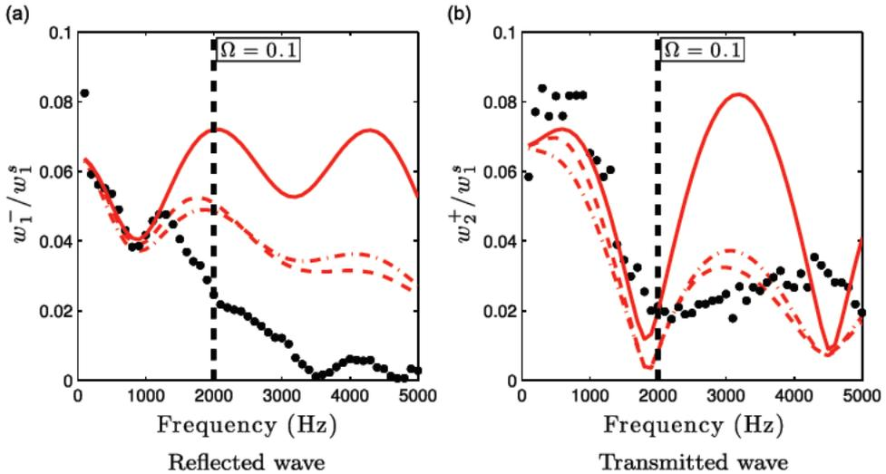
Fig. 9. Entropy transfer functions. —: Analytical theory without attenuation ; - - -: Analytical theory with attenuation extracted from the simulation ; · · · : Analytical theory with a simplified attenuation model ; ●: Numerical simulations.
