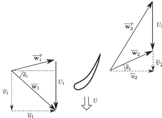
Fig. 2. Sketch of the flow through a rotor blade. Superscript ( $\prime$ ) represents the variables in the rotor reference frame.
