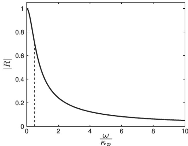
Fig. 5. Reflecting coefficient (—) of the outlet boundary condition. - - -: cutoff angular frequency  $\omega/\kappa_p = 0.5$ , leading to  $|R_{out}| = 1/\sqrt{2}$  (-3 dB). Below this limit,  $\omega/\kappa_p < 0.5$ , the boundary condition can be considered as fully reflecting.
