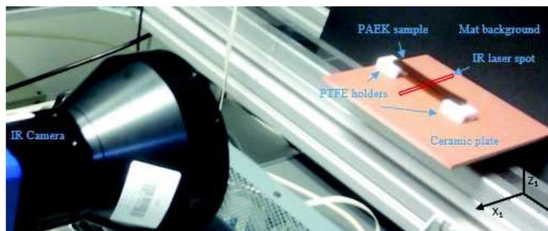
FIGURE 2: Layout of infrared recording scene
