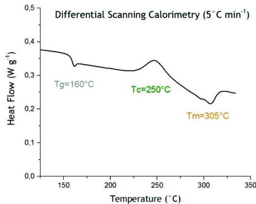
**FIGURE 5:** DSC thermogram of PAEK for the quasi-amorphous molded specimen
