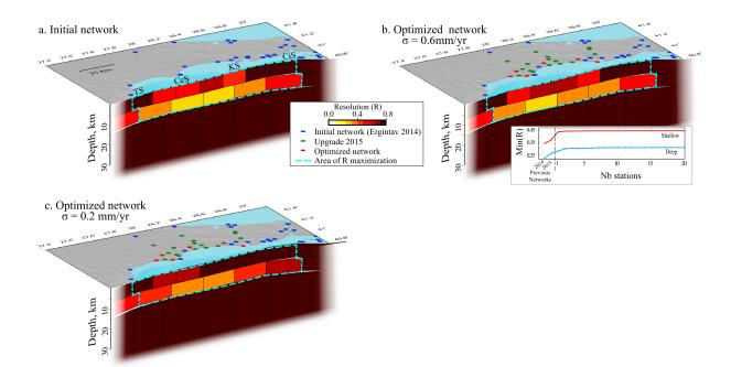
**Figure 3.** Model resolution of (a) the initial network; (b) the optimum network considering  $\sigma_d = 0.6$  mm/yr; (c) the optimum network assuming  $\sigma_d = 0.2$  mm/yr. The bottom right inset (Figure 3b) shows the minimum of resolution for each optimized row (area of maximization delimited by the dashed blue line) as function of the number of added stations.
