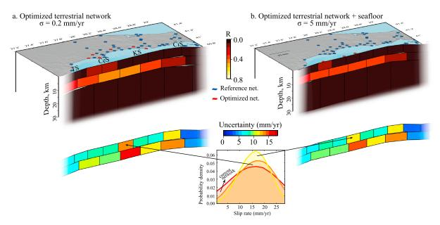
**Figure 4.** Model resolution compared to posterior  $2\sigma$  uncertainties (bottom) on slip rate for (a) the terrestrial network ( $\sigma_d = 0.2 \text{ mm/yr}$ ); (b) the network combining onland ( $\sigma_d = 0.2 \text{ mm/yr}$ ) and seafloor sites ( $\sigma_d = 5 \text{ mm/yr}$ ). The bottom inset shows slip rate marginal PDFs for the current network (red; Figure 2), the optimum terrestrial network (orange), and the optimum network including onland and seafloor sites (yellow).
