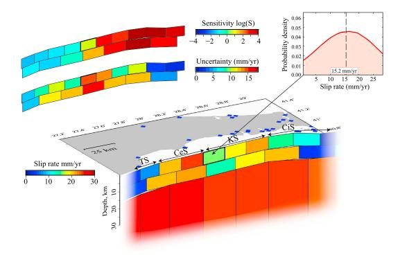
**Figure 2.** Posterior mean slip rate model (mm/yr). The top-left inset shows the slip sensitivity of the GPS network and the corresponding  $2\sigma$  posterior uncertainties. The top-right inset shows the marginal PDF of interseismic slip rate in the KS (patch highlighted by thicker contour).
