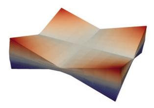
Fig. 4 Deformation envelope generated by all combinations of the reinforcement orientations of the top and bottom plies
