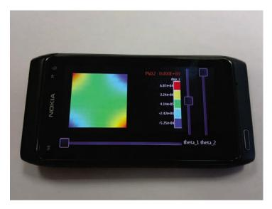
Fig. 3 Composite laminate analysis on a smartphone
