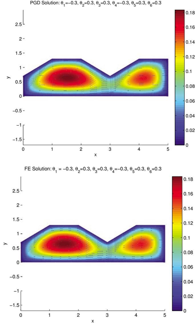
**Fig. 5** Comparing  $u(\mathbf{x}, \theta_1 = -0.3, \theta_2 = 0.3, \theta_3 = 0.3, \theta_4 = -0.3, \theta_5 = 0.3, \theta_6 = 0.3)$  with the finite element solution  $u(\mathbf{x})$ ,  $\mathbf{x} \in \Omega$ , with  $\Omega$  defined by  $\theta_1 = -0.3, \theta_2 = 0.3, \theta_3 = 0.3, \theta_4 = -0.3, \theta_5 = 0.3, \theta_6 = 0.3$ .
