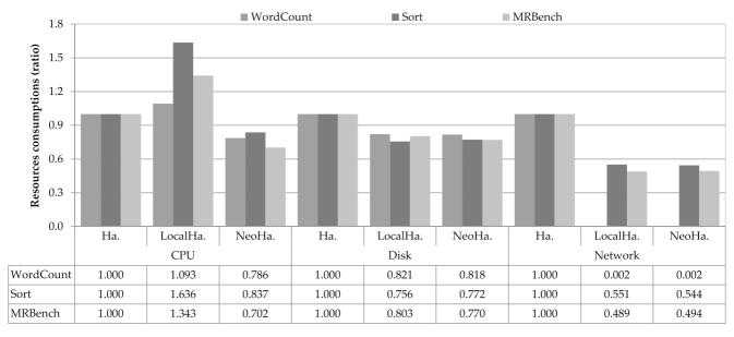
Fig. 6 The comparison of accumulative resource consumption (normalized by Hadoop) of three systems with WordCount, Sort and MRBench
