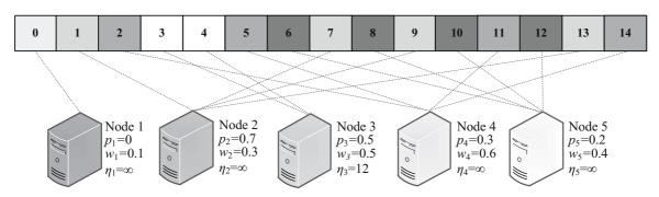
Fig. 1 An example of the modulo based DPA
