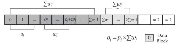
**Fig. 2** The data placement of  $f_0$ ' when the node  $c_i$  is added
