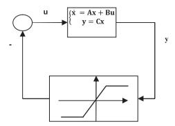
Fig. 4. Example 2: a general feedback interconnection of a saturating system.
