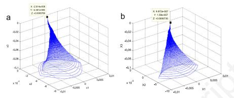
Fig. 6. Example 2: (a) trajectory for stabilization based on system states, (b) trajectory for stabilization based on estimated states.
