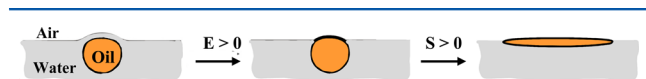
Figure 1. Scheme of the physical meaning of the entering coefficient, E . Adapted from ref 14.
