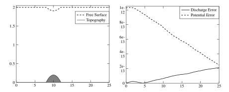
Fig. 1 Subcritical flow experiment. Left panel: free surface and topography for the steady state. Right panel: errors on the discharge q and the potential  $\Phi$ .
