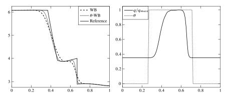
Fig. 2 Riemann problem at time t = 0.02s. Left panel: free surface. Right panel: value of  $\theta_i^n$  for the  $\theta$ -WB scheme.
