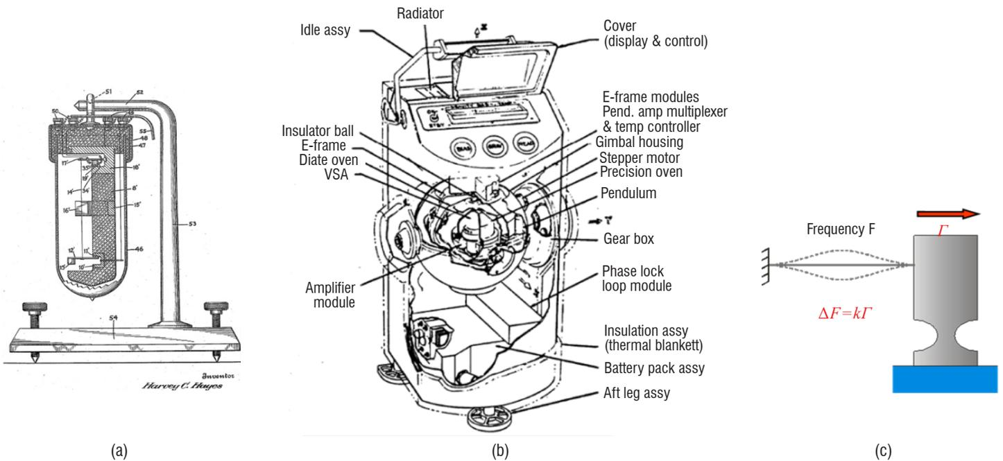
Figure 3 – (a) first vibrating string gravimeter proposed by H. C. Hayes in 1928, (b) lunar VSA gravimeter proposed by the Charles Stark Draper Laboratory for the Apollo 17 mission, (c) vibrating beam accelerometer, the string is changed by a beam in bending mode
