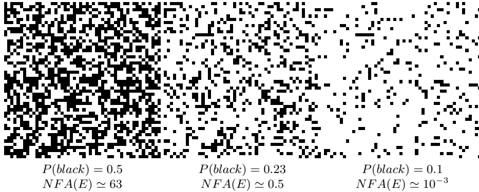
Fig. 3. Illustration of the number of false alarms. Unlike the more complex segments matching Definition 1, the events considered here are simply “perfectly horizontal segments”. The property associated to the event is the length and the a contrario random model is an image whose black pixel density is the same as in the original image but where points are spatially independent and uniformly distributed. A segment of 6-pixel length has been artificially added to each image, which otherwise follows the a contrario model. As the density of black pixels gets smaller, the number of false alarms of the 6-pixel segment decreases and it becomes an increasingly important deviation from the a contrario model. Our perception seems to follow similar rules: the segment becomes detectable with a NFA of 0.5 and obvious for a NFA of 10^{-3} .
