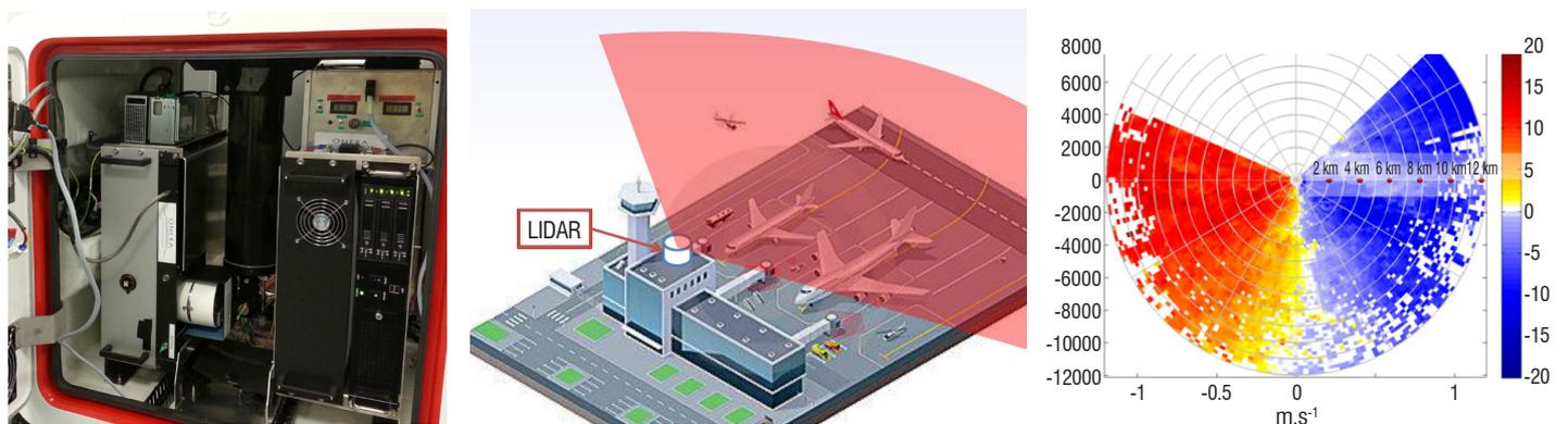
Figure 14 – left: ONERA high-power laser installed in the modified Windcube 200S<sup>®</sup>; middle: PPI scan for airport measurements; right: raw-wind data (radial wind speed) collected at Toulouse Blagnac airport. Data range up to 10 to 12 km
