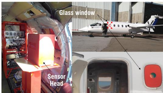
Figure 25 – AIM2 installed onboard a P180
