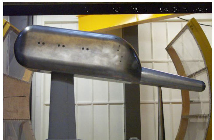
Figure 4 – Simplified blunt fuselage model in the test section of the wind-tunnel
