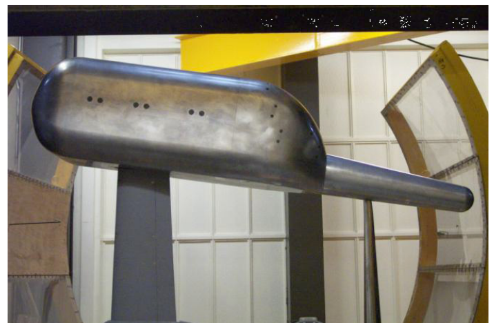
Figure 4 – Simplified blunt fuselage model in the test section of the wind-tunnel
