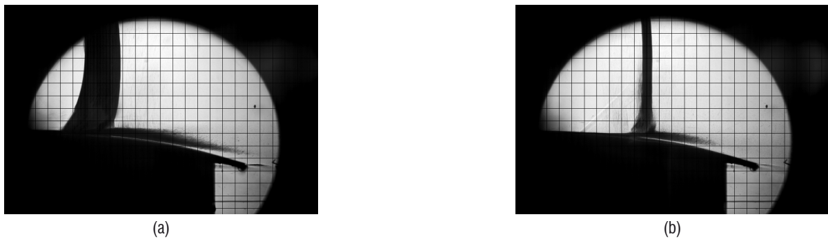
Figure 7 – Buffet at M_0 = 0.73 (supercritical airfoil OALT25) – Minimum intensity projection of the Schlieren movies for (M_0, \alpha) = (0.735, 4^\circ) : (a) forced transition cases (7%) and (b) natural transition cases, [17].
