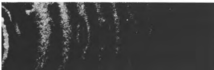
Fig. 5: Interference pattern of a 85 mm thick steelplate. Liquid-layer: waterfilm 2 mm high
