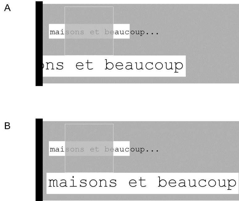
Fig 6. Example of ROAV adaptation to a monitor's screen border. The grey rectangle represents a portion of the screen delimited by the left screen border (vertical black bar). A/ this shows what would happen if the ROAV location was determined without taking into account the presence of the screen border: the first five letters of the word "maisons" would be invisible. B/ To allow full visibility of the ROAV, the mapping rule adjusts the ROAV location by aligning its left border with the left screen border.
