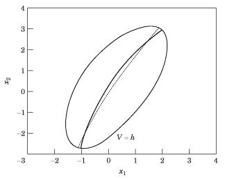
Figure 13. The first mode:  $x_1$  versus  $x_2$ . The dashed curve represents the eigenvectors in each of the linear regions. Note that the bilinear frequency is a better approximation than the mode shape. —, Non-linear normal mode;  $\cdots$ , bilinear mode shape.
