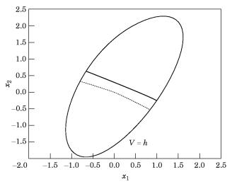
Figure 15. The second mode:  $x_1$  versus  $x_2$ . The dashed curve represents the eigenvectors in each of the linear regions. Note that the bilinear frequency is a better approximation than the mode shape. —, Non-linear normal mode,  $\cdots$ , bilinear mode shape.
