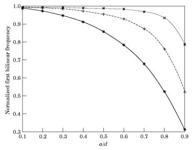
Figure 7. The variation of the first bilinear frequency with crack depth, where b is the location of the crack and L is the length of the beam. \*, b/L = 0.2; +, 0.5; ×, 0.7.
