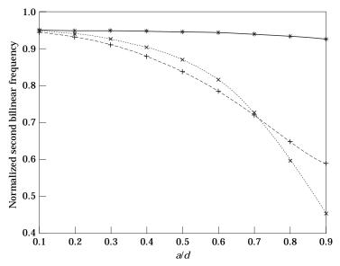
Figure 8. The variation of the second bilinear frequency with crack depth, where b is the location of the crack and L is the length of the beam. \*, b/L = 0.2; +, 0.5; ×, 0.7.
