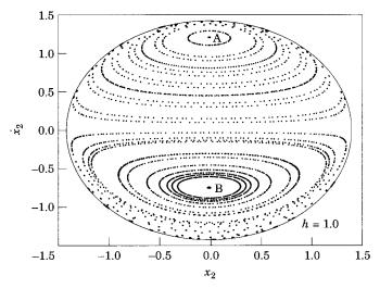
Figure 20. The Poincaré map for  $k_2 = 0.0$ , h = 1.0 and surface of section  $x_1 = 0$ ,  $\dot{x}_1 > 0$ . This figure corresponds to a linear system; in contrast to Figure 18, which corresponds to a piecewise-linear system: h is the total energy of the system.
