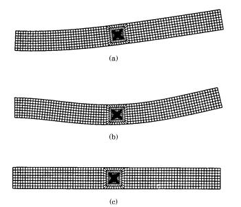
Figure 6. Constrained mode shapes for the (a) first, (b) second and (c) third mode shapes.
