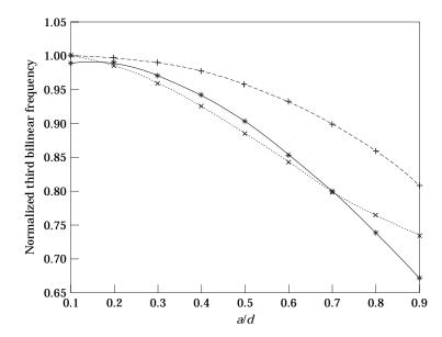
Figure 9. The variation of the third bilinear frequency with crack depth, where b is the location of the crack and L is the length of the beam. \*, b/L = 0.2; +, 0.5; ×, 0.7.
