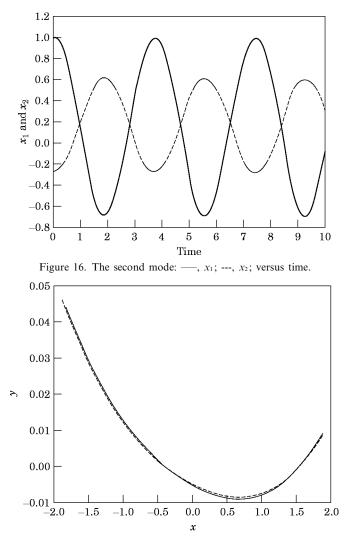
Figure 17. A comparison of the numerical integration and perturbation methods:  $k_2 = 0.1$ . —, Numerical integration; ---, perturbation method.
