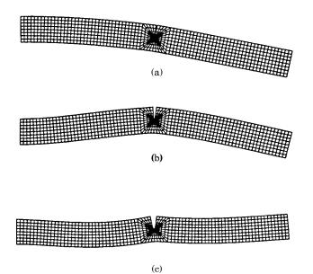
Figure 5. Unconstrained mode shapes for the (a) first, (b) second and (c) third mode shapes.
