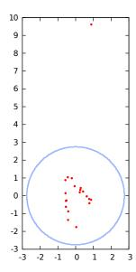
Figure 4. After the robust Principal Component Analysis, the point cloud corresponding to the non-falsified sub-images are grouped in a disc shape. The outlier, in the top can be detected with a  $\sigma$ -clipping.
