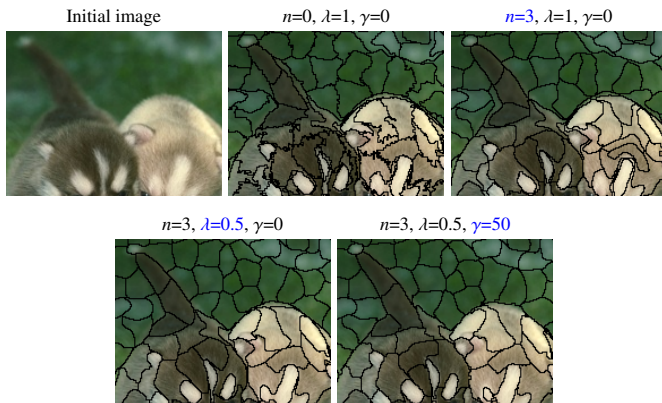
Fig. 12. Visual impact of the distance parameters. Each contribution progressively increases the decomposition accuracy by adding more relevant features.
