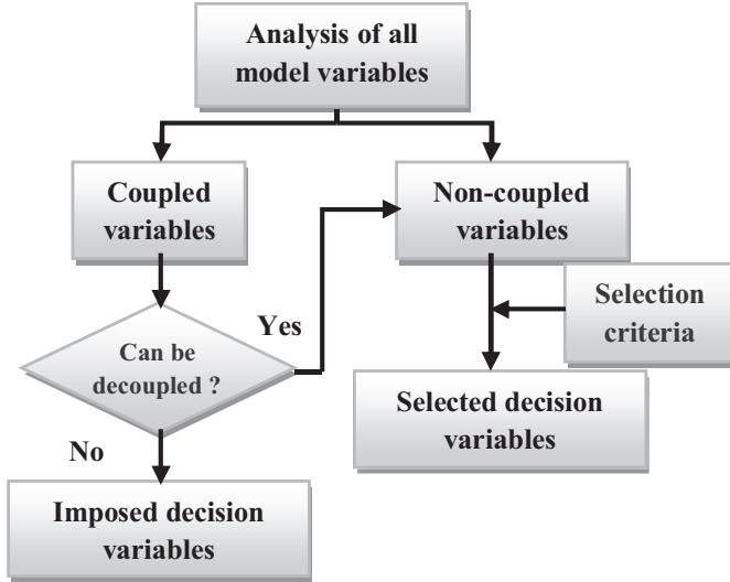
Fig. 6. Selection method algorithm.
