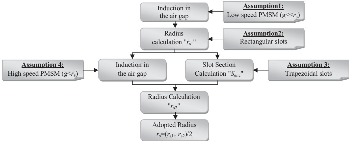
Fig. 10. Radius calculation steps involving implicit blocks.
