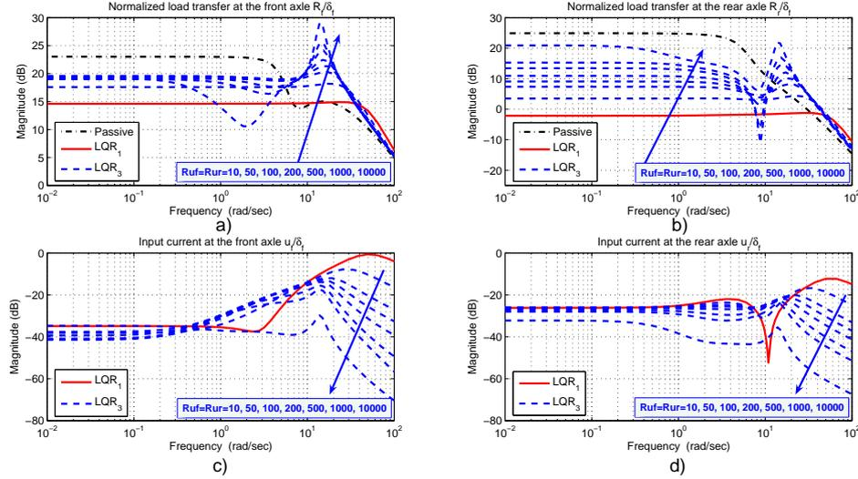
Figure 6. Case 2, transfer functions magnitude of (a, b) normalized load transfers ( $\frac{R_{f,r}}{\delta_f}$ ) and (c, d) input currents ( $\frac{u_{f,r}}{\delta_f}$ ) at the axles.
