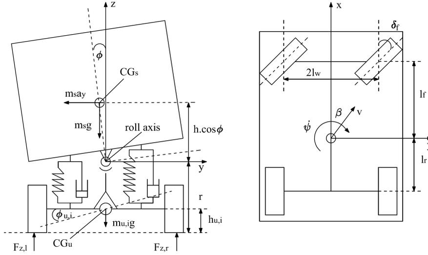
Figure 2. Yaw-Roll model of single unit heavy vehicle [4].
