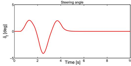
Figure 7. Time responses of steering angle  $\delta_f$  [4].
