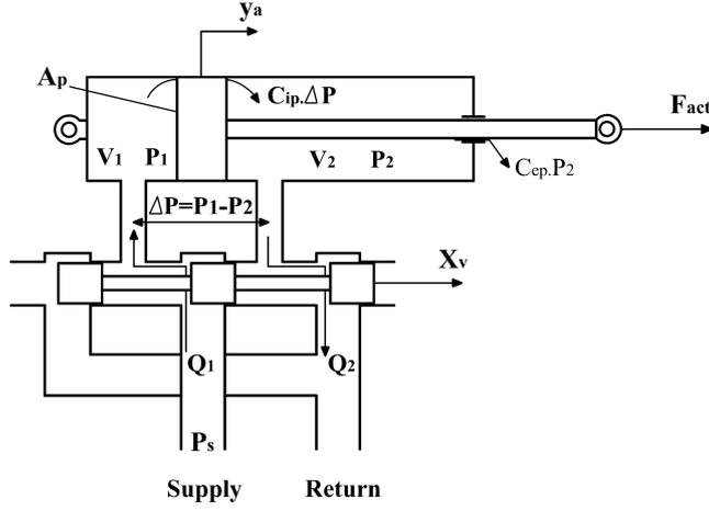
Figure 1. Diagram of the electronic servo-valve hydraulic actuator [17].
