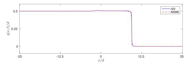
**Figure 5.** Propagation of a shock wave for the regularisation parameter  $\varepsilon = 10^{-2}$ . A little wavelet travelling leftwards is due to the fact that the initial condition is chosen to be a smoothed shock wave profile (instead of being a sharp HEAVISIDE function).
