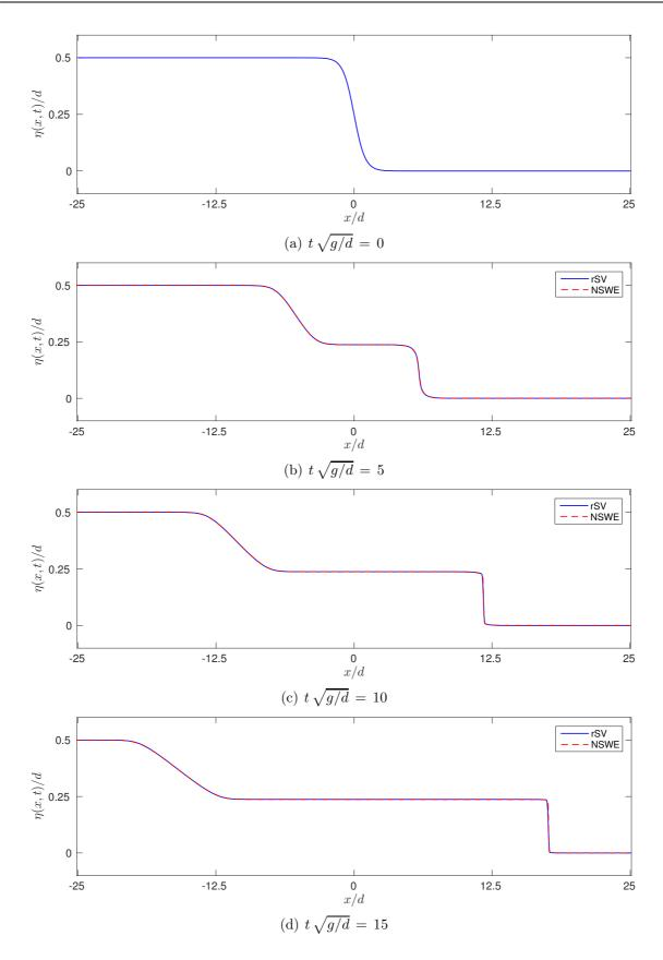
**Figure 2.** Dam break problem solved with the hyperbolic and regularised models. The common initial condition is shown on the upper panel (regularisation parameter  $\varepsilon = 10^{-3}$ ).
