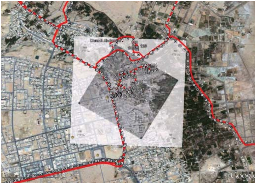
Fig. 10. Superimposition of the 1948 ortophoto and the 2010 topographic survey on an Ikonos Google high resolution image
