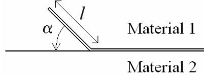
Figure 1. Crack kinking out of an interface.
