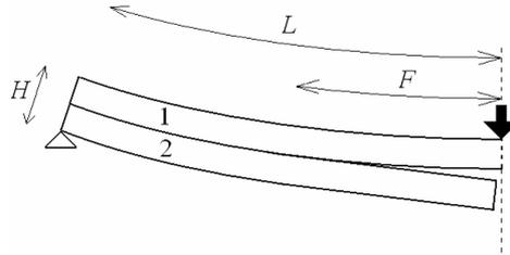
Figure 2. 3-point bending test,  $F/L = 0.25$ ,  $H/L = 0.2$  (1/2 specimen).
